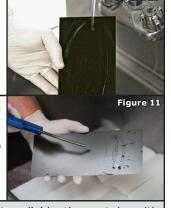
**TECH TIP:** Alternate your brush strokes & direction every 10 to 15 seconds and brush the entire cliché surface. Staying in one area will create an uneven depth of the etch.
