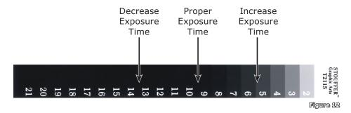
Look at the test cliché to see the step pattern that has been etched. If the exposure time you selected (example was 180 seconds) is correct, the step will show a value between 9 and 10 on the scale. If the correct value is not found, use the attached calibration chart to properly calibrate the exposure by increasing or decreasing exposure time.
