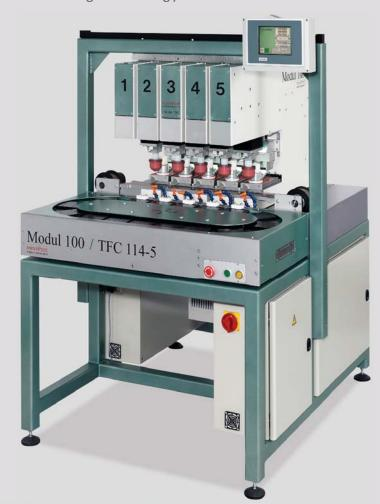
machines in the **MODUL SERIES** and they are perfectly suited for high speed printing on small objects such as; golf balls, USB memory sticks, cell phone bodies & lenses, saw blades, pens, lighters, coins, surgical devices, electronic connectors and much more. The **MODUL SERIES** of machines are available with as many colors (print heads) as you need for your product decoration... The sky is the limit with this completely modular approach to system design.
